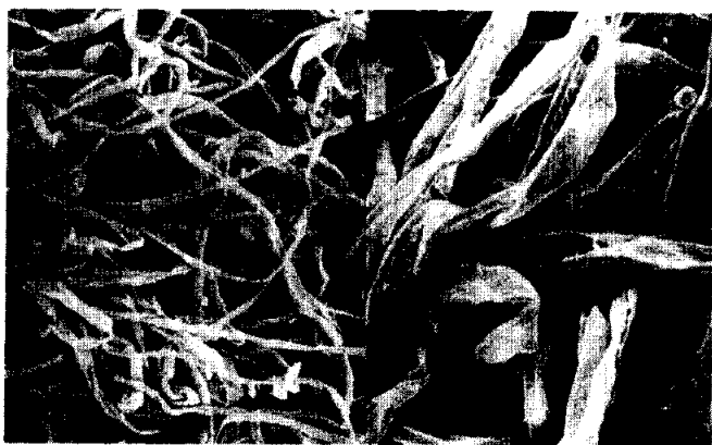
Figure 2 – Dyed nep composed of immature fibres on fabric dyed with C.I. Direct Red 23; left 105 \times , right 350 \times
