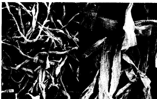
Figure 5 – Dyed nep composed of torn mature fibres on fabric dyed with C.I. Direct Black 80; left 105 \times , right 350 \times
