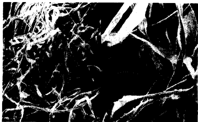
Figure 3 – Dyed nep composed of both dead and immature fibres on fabric dyed with C.I. Direct Red 23; left 105 \times , right 350 \times
