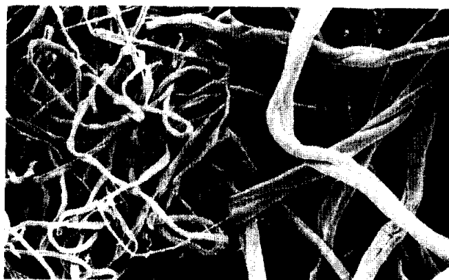
Figure 4 – Dyed nep composed of thin, mature fibres on fabric dyed with C.I. Direct Black 80; left 105 \times , right 350 \times
