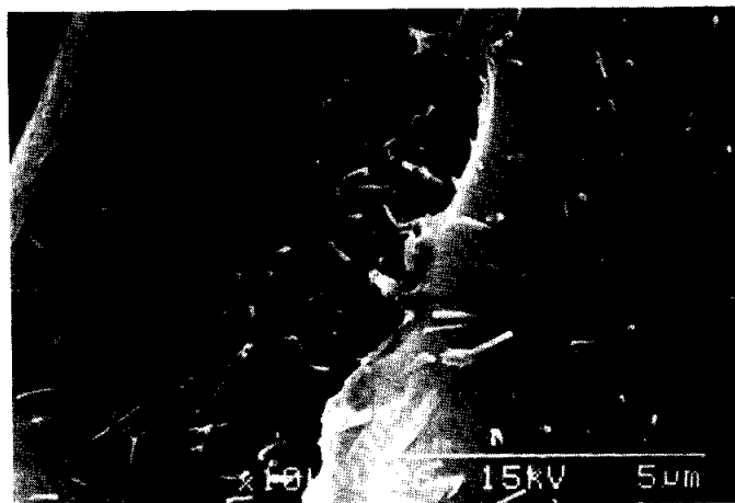
Figure 6 Dye particles on white cloth stained with Blue BB; dye content ( x ) 9.57 \times 10^{-7} mol/g, number of rubs ( t ) 200, applied weight ( W ) 400 g
