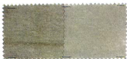
FIG. 2— Effect of faulty singeing before carrier and pad-thermofix dyeing on Terylene-cotton fabric
